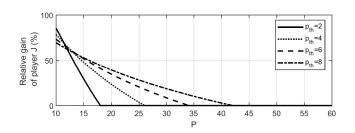
Fig. 4. Relative gain of player J, evaluated by function E, for different values of  $p_{\rm th}$  for N=10,  $\sigma_J^2=1$  and  $\Gamma=4$ .
