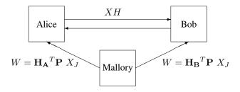
Fig. 1. Alice and Bob have single transmit and receive antennas and exchange pilot signals X over a Rayleigh fading channel with realization H. A MiM, Mallory, with multiple transmit antennas can inject a suitably pre-coded signal  $\mathbf{P}X_J$ , such that the received signal at both Alice and Bob coincide  $W = \mathbf{H_A}^T \mathbf{P} = \mathbf{H_B}^T \mathbf{P}$ .
